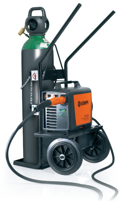
FitWeld 300 mounted on ST7 transport unit.
